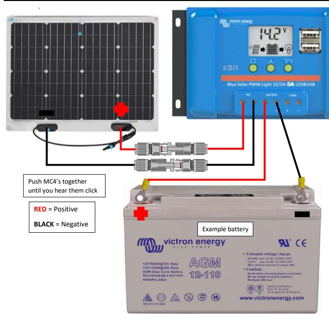
Connect the battery cables first, then the solar.
